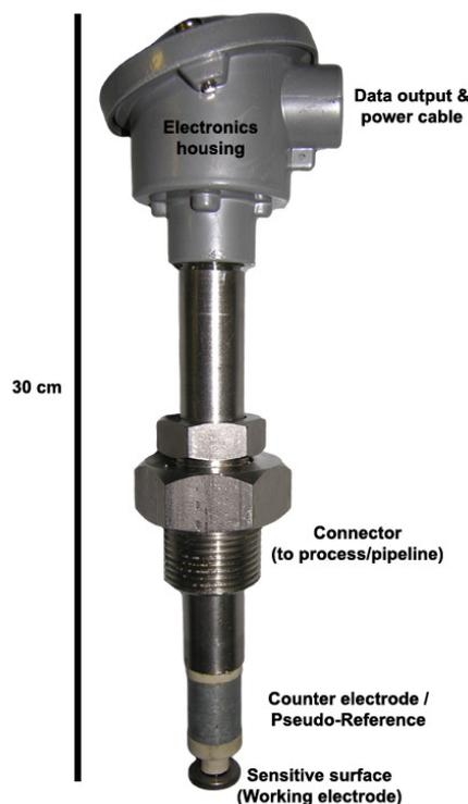
**Fig. 2** – ALVIM biosensor.
