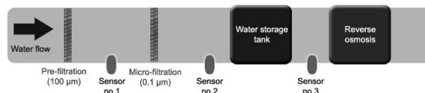
**Fig. 3** – Scheme of FISIA – Italmipianti reverse-osmosis desalination plant and ALVIM probes disposition.
