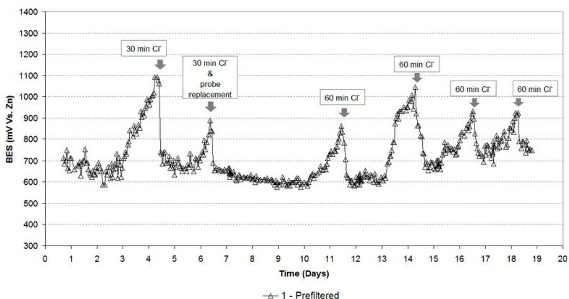
**Fig. 7** – ALVIM probe BES evolution (mV Vs. Zn) during the use of ALVIM system as a chlorination triggering device. The arrows mark pipeline chemical cleaning by means of water chlorination (1 ppm) at the intake.
