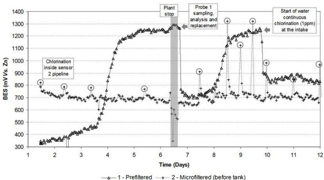
**Fig. 6** – ALVIM probes BES evolution (mV Vs. Zn) during the second test in a pilot reverse-osmosis desalination plant. The circles mark chlorinations in the section between MF and water storage tank. The gray area marks plant stop for maintenance. The arrow on day 6 marks sensitive surface no.1 sampling, analysis and replacement. The arrow on day 9 marks the start of continuous chlorination (1 ppm) at the intake (whole pipeline treatment).
