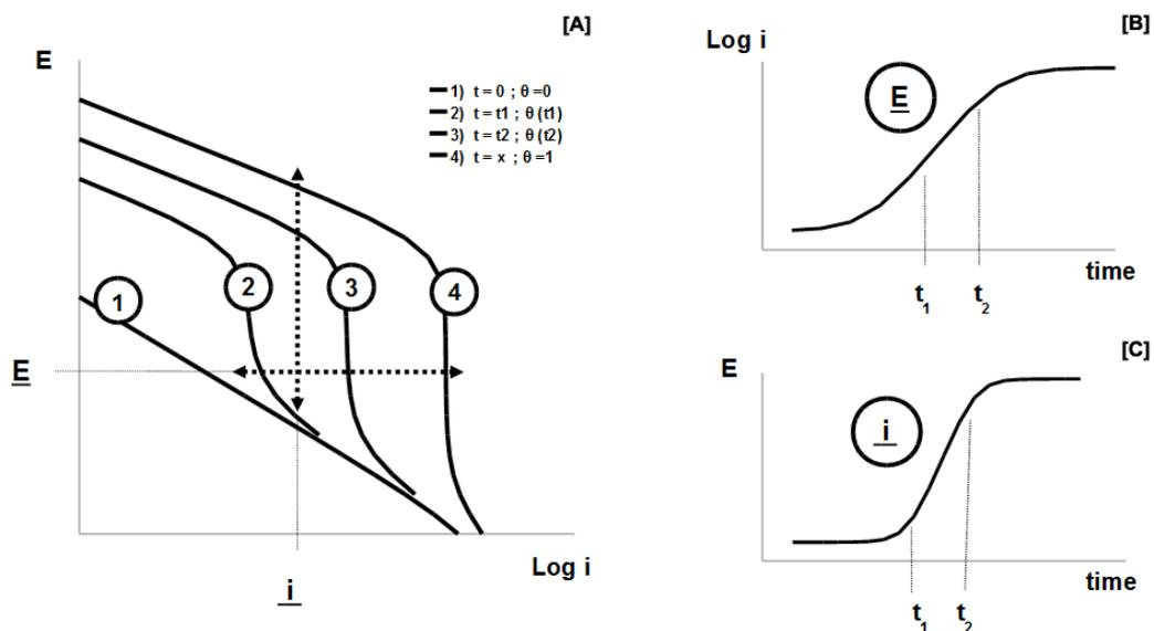
**Fig. 1** – Evolution of the overall cathodic curve (current  $i$  versus potential  $E$ ) during the gradual development of biofilm on a stainless steel surface [A], cathodic currents measured at a fixed potential  $\underline{E}$  [B] and potentials measured at a fixed cathodic current  $\underline{i}$  [C] during biofilm growth.
