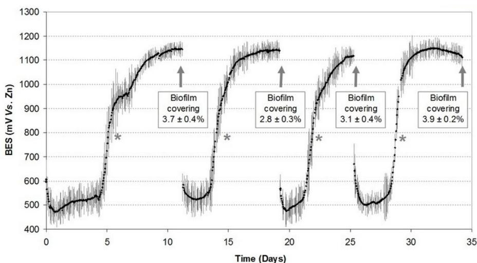
**Fig. 4** – ALVIM probes BES evolution (mean ± SE, mV Vs. Zn) during preliminary testing in a tank with constantly renewed natural seawater. The asterisks mark the reaching of the chosen biofilm covering threshold (1% of the WE), the arrows mark sensitive surface sampling/analysis (biofilm covering data are indicated in the boxes, as % ± SE, calculated on the three replications) and replacement.
