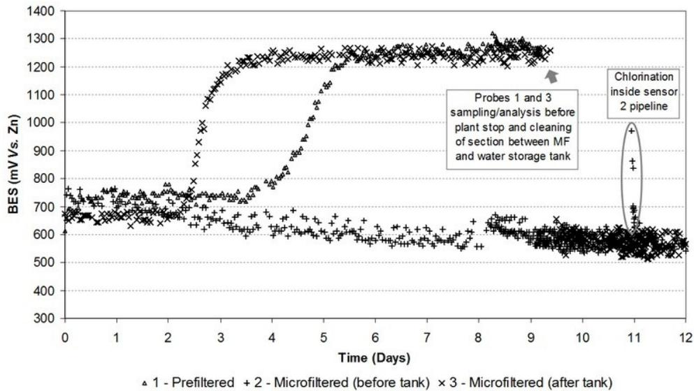
**Fig. 5** – ALVIM probes BES evolution (mV Vs. Zn) during the first test in a pilot reverse-osmosis desalination plant. The arrow marks sensitive surfaces no.1 and no.3 sampling/analysis before plant stop and cleaning of the section between MF and water storage tank; on sensor no.3 a new sensitive surface was installed. The oval marks a chlorination in the same pipeline.
