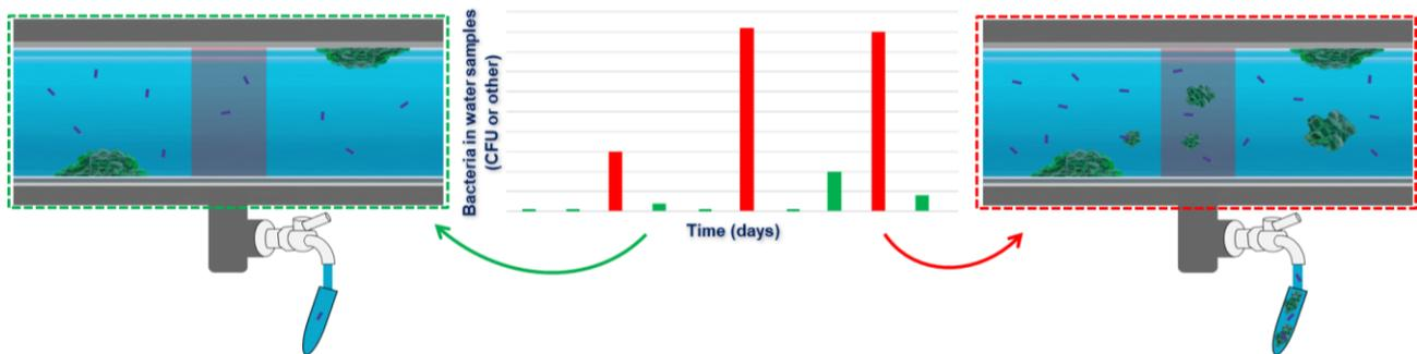
Figure 4: A biofilm contamination can lead to high and sudden spikes of bacteria in the liquid
