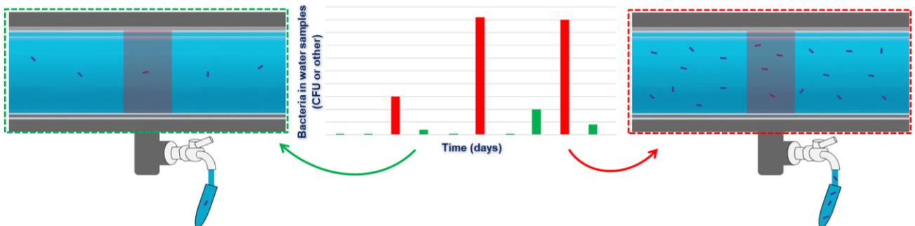
Figure 2: Large and unexpected fluctuations in bacterial count are commonly attributed to microorganisms entering the process with feedwater
