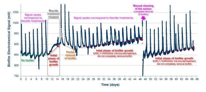
The ALVIM Sensor provided a precise, early-warning indication of biofilm growth, that underlined the need of an additional, stronger sanitation treatment, to be applied at least occasionally. This case
